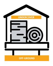
**Storing materials off-ground** does not require chemical treatment. However, materials must be covered at all times with a tarpaulin, or be stored inside a shed.
