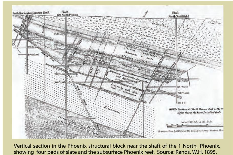
Vertical section in the Phoenix structural block near the shaft of the 1 North Phoenix, showing four beds of slate and the subsurface Phoenix reef. Source: Rands, W.H. 1895.
