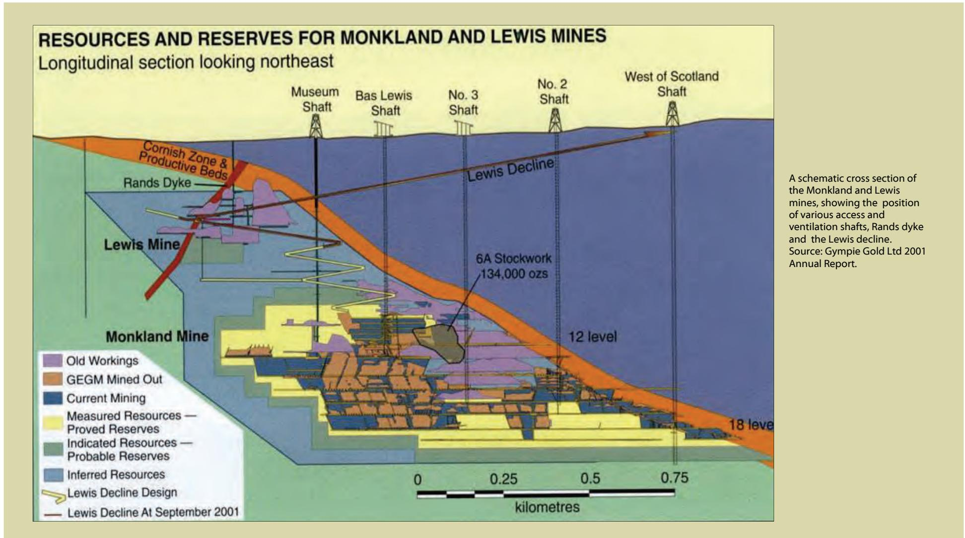
A schematic cross section of the Monkland and Lewis mines, showing the position of various access and ventilation shafts, Rands dyke and the Lewis decline. Source: Gympie Gold Ltd 2001 Annual Report.
