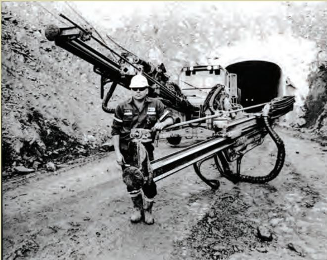
"Jumbo" Mine drilling rig on the Lewis decline at the entrance portal to the Lewis mine.
