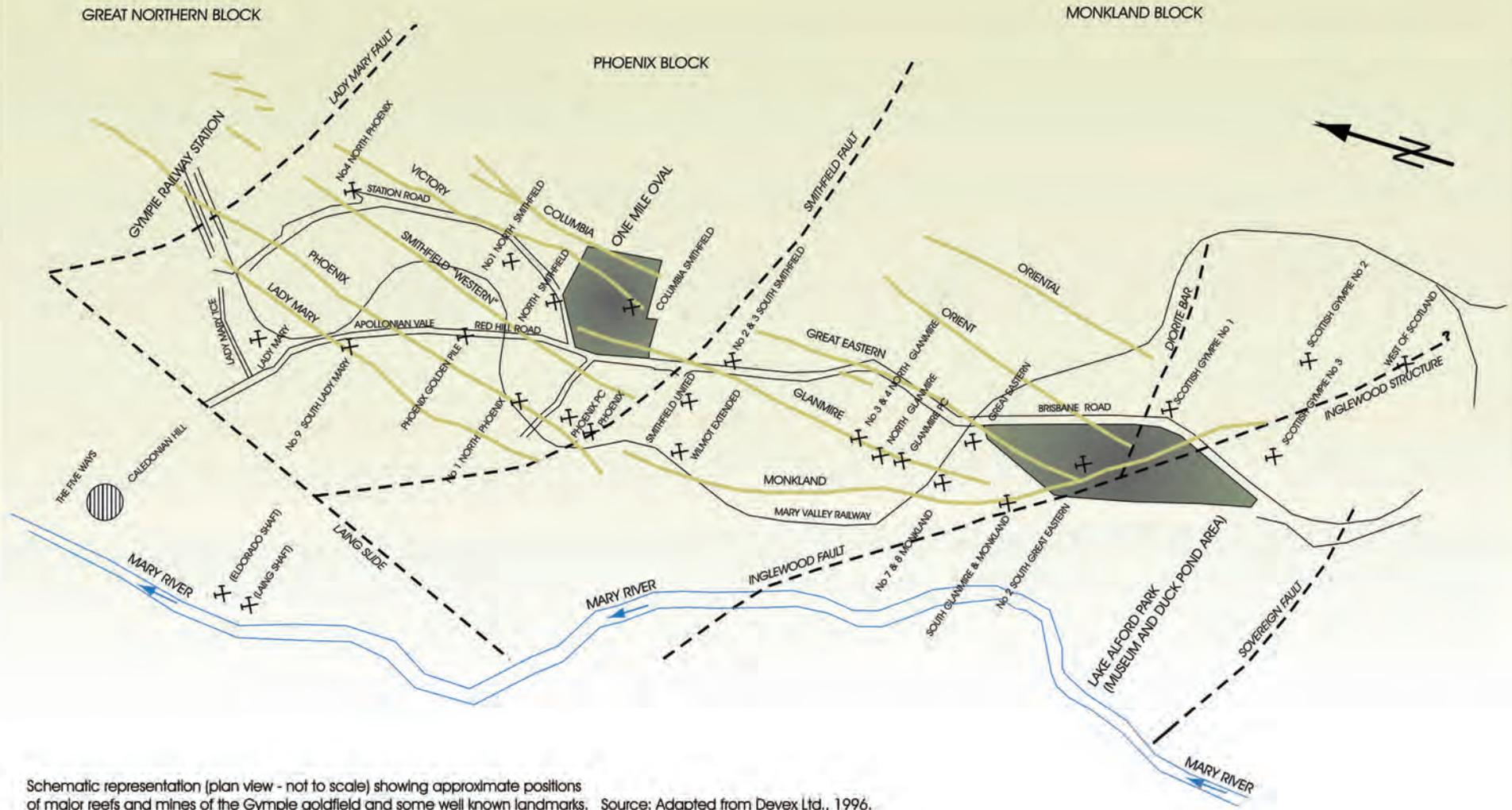
Schematic representation (plan view - not to scale) showing approximate positions of major reefs and mines of the Gympie goldfield and some well known landmarks. Source: Adapted from Devex Ltd., 1996.
