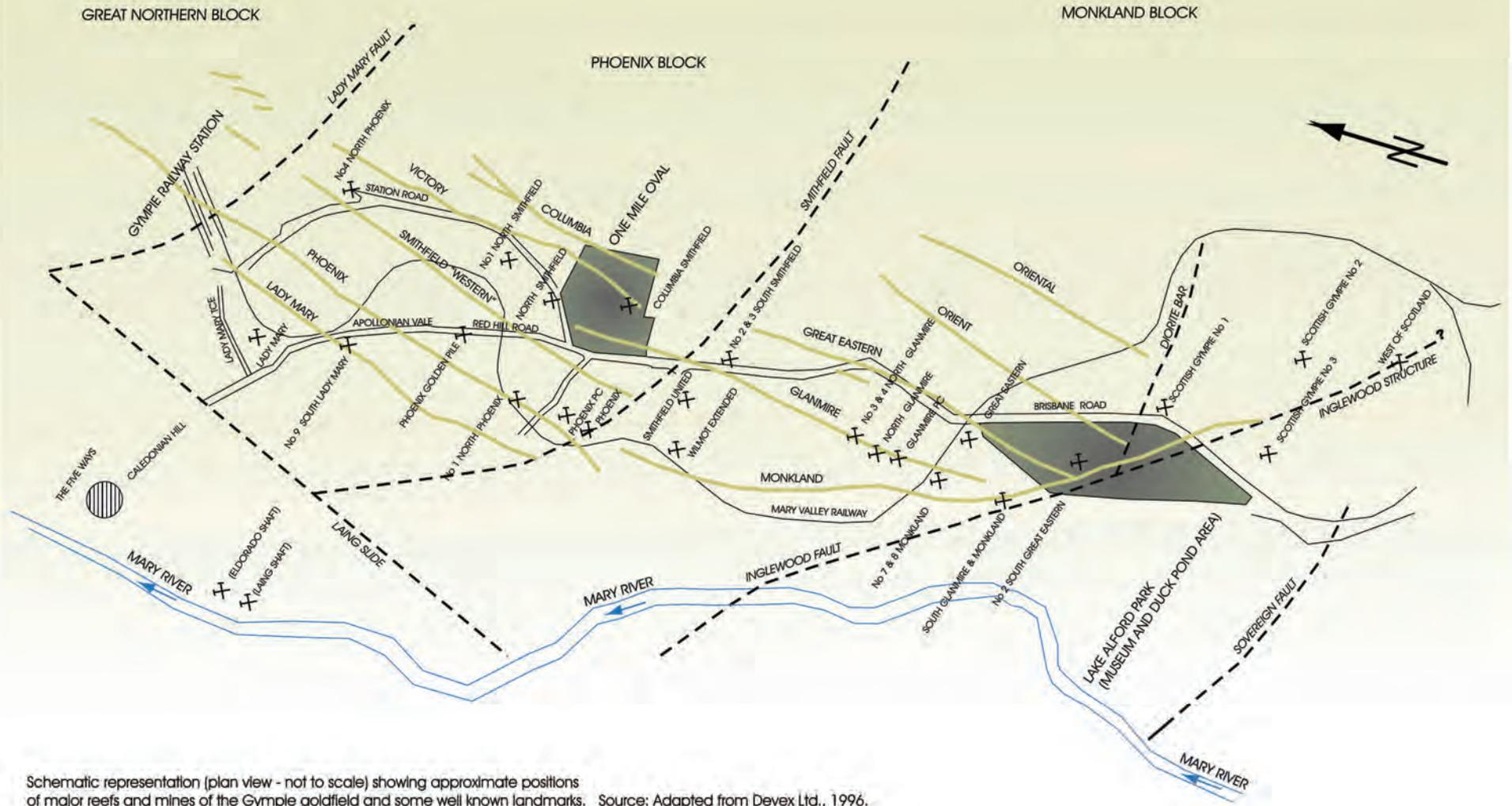
Schematic representation (plan view - not to scale) showing approximate positions of major reefs and mines of the Gympie goldfield and some well known landmarks. Source: Adapted from Devex Ltd., 1996.
