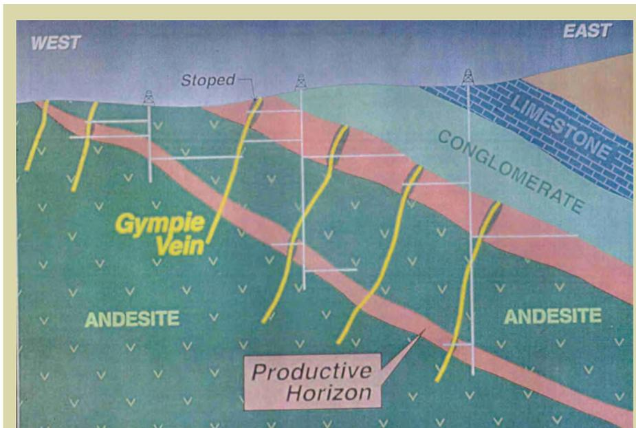
Schematic representation of the dip of the productive beds to the east, showing the resultant deepening of shafts and cross cuts in the exploration for gold bearing reefs.
