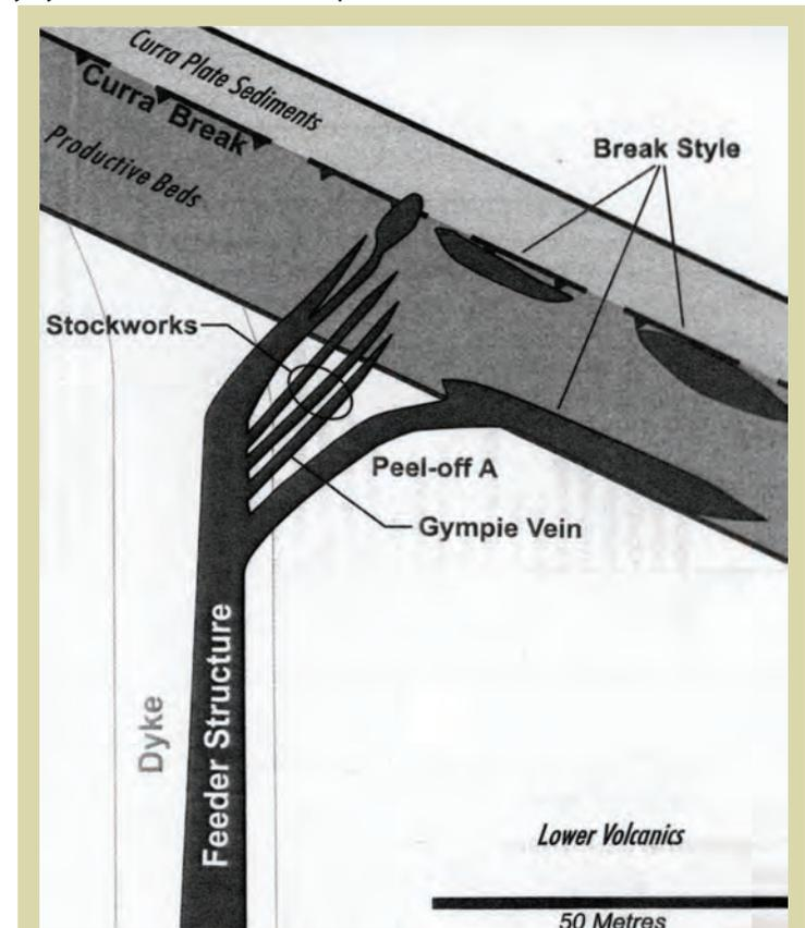
Schematic vertical representation of the Inglewood feeder structure within the Monkland structural block and the resultant ore bodies. Source: Buka Gold Ltd. Prospectus 2005.
